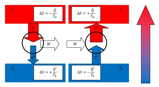
Fig. 2.11: Coupling of reversible generator and reversible heat pump, assuming different efficiencies
