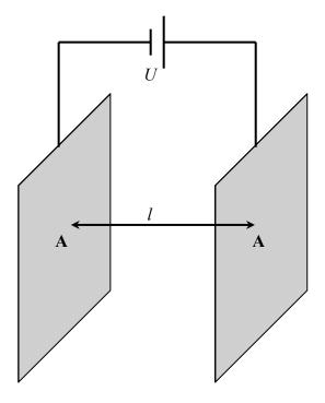
Figure 4.2: schematic presentation of an electrochemical cell
