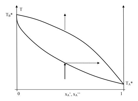
Fig. 2.22: Isobar boiling curve of an ideal binary mixture, and the principle of distillation
