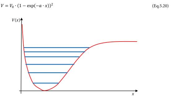
Figure 5.15: Morse potential and resulting energy levels
