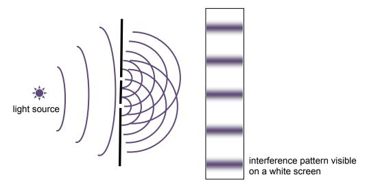
Figure 5.5: Diffraction of light wave on a two-slit setup
