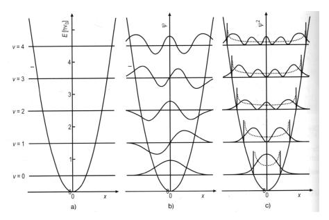
**Figure 5.14:** energy Eigenvalues (a)), wave functions (b)), and squared amplitudes (c)) of the harmonic oscillator (c) dotted lines = classical probabilities) (from: Gerd Wedler und Hans-Joachim Freund, Lehrbuch der Physikalische Chemie, p. 548, 6.Auflage, Weinheim 2012. *Copyright Wiley-VCH Verlag GmbH & Co. KGaA. Reproduced with permission.*)
