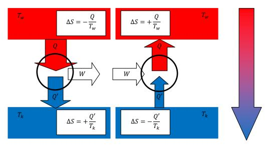
**Fig. 2.12:** Coupling of two processes, one reversible the other irreversible, always leading to spontaneous heat exchange, i.e. heat flowing from the hot to the cold reservoir.
