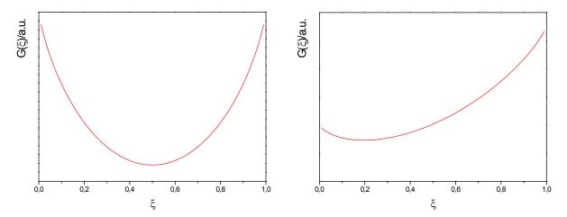
Fig. 2.32: Reaction free enthalpy versus conversion and the chemical equilibrium
